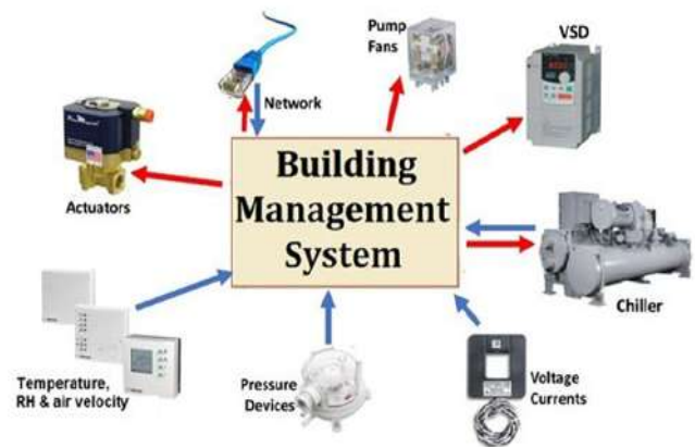
Figure 1 (Building Management system) Source- https://www.indiamart.com/proddetail/building-management-hvac-system
