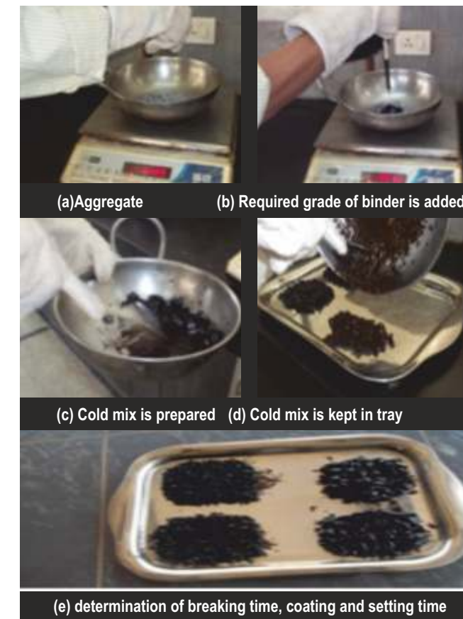
Figure 2 Mix Design of Cold Mix for Rural Roads
